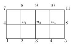
The general difference equation at  $(x_i, y_j)$  (five-point stencil for  $-\Delta$ )<sup>33</sup>:
