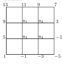
First, the values of u at the boundary nodes are calculated. Second, equations at the inner nodes are inferred. Finite difference equation at  $(x_i, y_j)$  is given by the five-point stencil:
