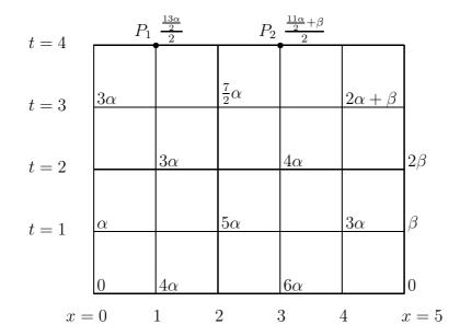
The points  $P_1$ ,  $P_2$  have to coincide with two mesh nodes. Since their x-coordinates are equal to 1 and 3, we conclude that the largest h we can consider is equal to one. The stability condition  $\tau \leq h^2/(2a^2)$ , where  $a^2 = \frac{1}{2}$ , then implies  $\tau \leq 1$ . Our choice: h = 1,  $\tau = 1$ .
